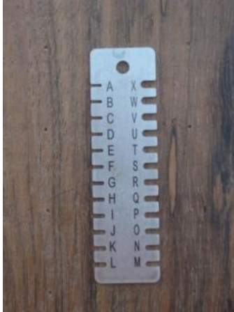
Figure 29. Hummingbird Tarsus Gauge: A tool to measure the long (widest) axis of the tarsus and aid in determining band size (photos: Lee Rogers and Anthony Hill).
